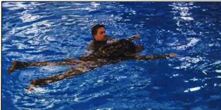
Fig.3. Test subject 1, Face down in the water for the self-righting test with subject 2 in the water manually operating the inflation system.
