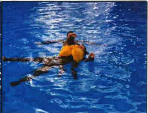
Fig.4. Test subject 1, self-righting successfully returned to a face up position (airways clear).
